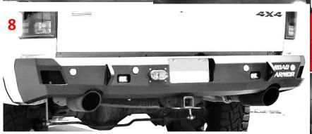
Install the bumper mounting bracket onto the frame using the supplied bolt kit
