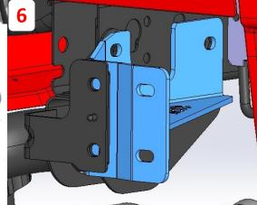
**Note** If truck has air pump option, it will need to be removed, and remounted on the new bracket
