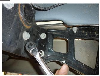
NOTE: Bumper will be removed during this step. Be prepared to hold bumper in place and remove once bolt plates are removed.
