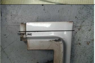
7. Remove plastic trims from lower front of guards. At the indicated cut line (along the moulded feature line approx. 23mm from top face) cut and retain the lower section of these trims. Deburr, if necessary touch up and refit the trims.
