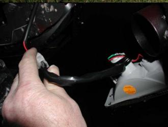
36. Wire up the indicator and clearance lamp assemblies. Use scotch locks to splice cables to existing indicator and clearance lamp wiring and cable tie securely.
