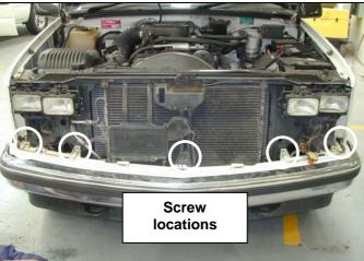
4. Remove plastic trim, this is secured by five screws located as shown.
