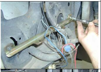
15. Fit grille outboard anchoring brackets as shown using existing screws.
