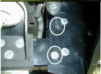
34. Drill and pin the bar to the mounts in 2 x places per side using M10 drill bit, as shown, then bolt up using M10 x 30 SEMS bolts and flange nuts.
