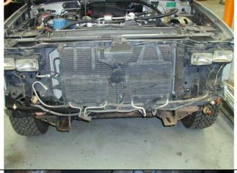
5. Remove bumper. Undo any electrical connections to lights in bumper. Undo two bolts per side retaining the bumper stabilising bars to the chassis. Loosen only the two bolts securing the stabiliser bars to the bumper, the bars should now be able to swing away from chassis. Undo the three bolts per side securing the bumper mount brackets to the chassis. Remove bumper.
