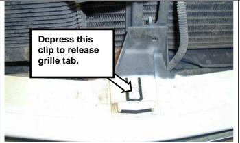
3. Showing clip detail, note that you may need a large flat blade screwdriver to reach the middle clip while reaching behind grille.
