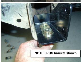
NOTE: IF THE CHASSIS IS 2500/3500 THEN FIT ADDITIONAL BRACKETS AS SHOWN IN STEPS 8 & 9, OTHERWISE PROCEED TO STEP 10.
