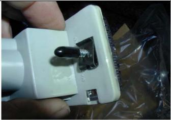
19. Remove lights from cartons and then remove screws and speed nuts from each light.
