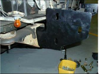
11. Position the nut plates with three M12 nuts fitted into chassis brackets, so that all holes line up with existing bumper mount holes in outboard side of chassis. Fit three M12 x 40 bolt and washer sets per side. Do up finger tight only
