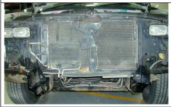
Slide mount brackets into chassis ends oriented as shown with large flanges outboard.
