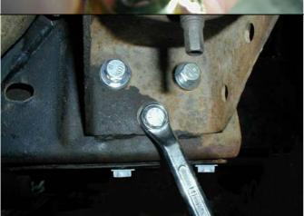
13. Nip up all bolts, check that the brackets are parallel to each other and the front edge of bracket flange is vertical, if not adjust and retighten.
