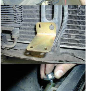
16. Fit grille centre anchoring bracket as shown using existing screw.
