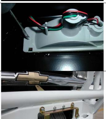
21. Fit lights using screws supplied in fitting kit, taking note of RH and LH light bodies, they are different, marked LH or RH and must be placed on the correct side of bull bar (drain holes down).
