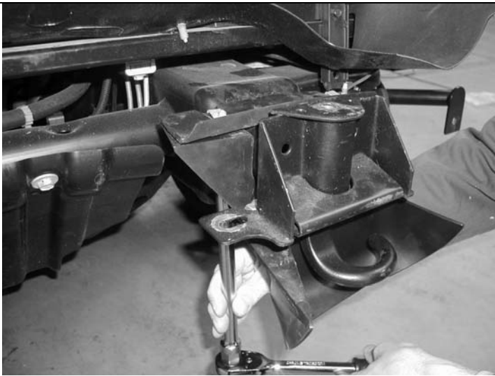
1.5 Remove plastic shrouds around chassis
