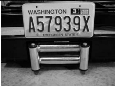
Fitting with winch, number plate above RFL
