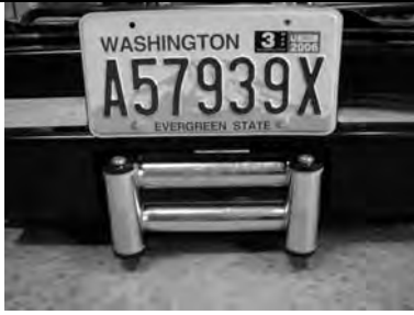
Fitting with winch, number plate above RFL
