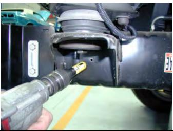
9. Use the Dia 19.0 hole saw, as shown, with 7.0mm hole as a guide to drill a hole through outer wall of chassis.
