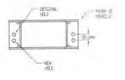
30. In some cases, the roller fair lead bracket must have a second set of holes drilled to line up with holes in winch bracket. If required, mark out as shown and using a 13.0 mm drill bit, drill two holes as shown in diagram.
