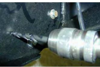
42. Using the M10 pilot holes in mount brackets, drill pinning hole through uprights on bull bar. Fit M10 screw, washer set and flange nut and do up tight.
