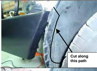
55. Trim fender liner with air hacksaw or similar tool along line as shown. Cut away the outboard flap, which normally fits in the end of the bumper wing. This is so the liner can be held back easily by the retaining bracket at step 56.
