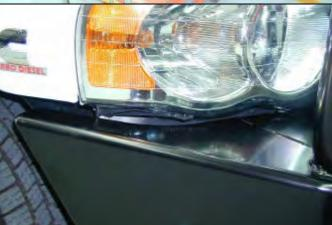
40. Bolt the bar to the mounts using M12 bolts, large flat washers and spring washers. Bolt the bar to the mounts using M12 bolts, large flat washers and spring washers. Align the bar to the profile of the guards, grille and light profile and tighten all bolts.
