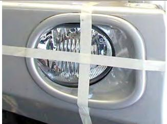
52. Use adhesive tape to secure plastic mold while Sikaflex cures.
