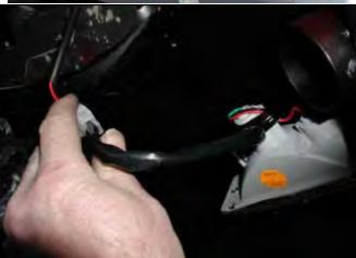
53. Wire up indicators and running lamps. Wire loom extensions are supplied in fitting kit.
