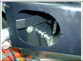
41. When bar is aligned, tighten bolts.
