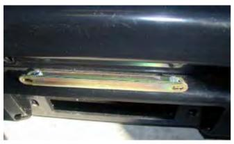
Secure the number plate bracket using M6 bolts, flat washers and flange nuts.Attach the longer side to the bullbar and the shorter side to the number plate.
