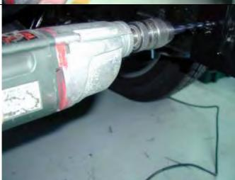
10. Then, as shown, using a Dia 10.0 drill, drill hole through inner wall of chassis.
