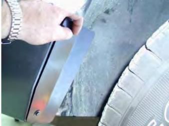
56. Fit liner retainer bracket with black M6 bolt and washer sets into M6 cage nuts in wing returns each side as shown.
