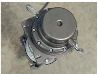
Note: As supplied from Warn, the winch handle on 1500 and 16500lb winches should be in the position as shown. This is correct orientation for this bar.
