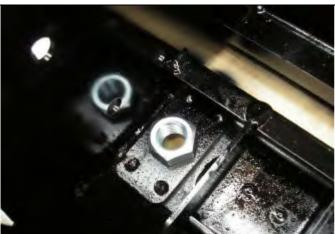
22. Fit large eyebolt nut into the plate on the inside of the bar.
