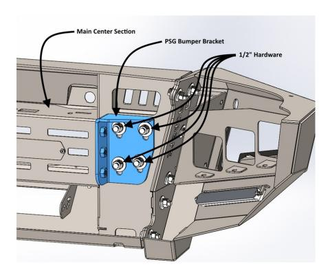
\*\*NOTE: Be sure to remove grille assembly prior to installing iD front bumper. Doing so will allow easy access to kit ½" bumper bracket bolts during installation.\*\*
