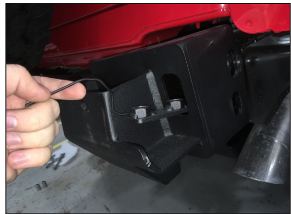
10. Install right bracket (pos. 3) on the vehicle frame, put insert bracket M12 (pos.U) onto the frame through the bracket hole. Attach the bracket to the Insert bracket M12(pos. U) using bolts M12x30 (pos.E) and washers 12 (pos.J). Do not tighten yet.
