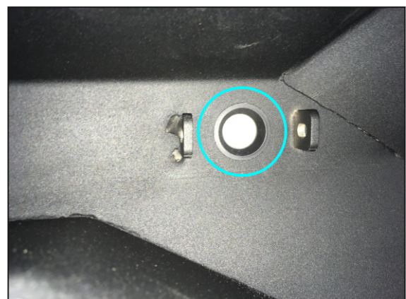
30. Install parking sensor washers (pos. L) into the holes that you hammered out.
