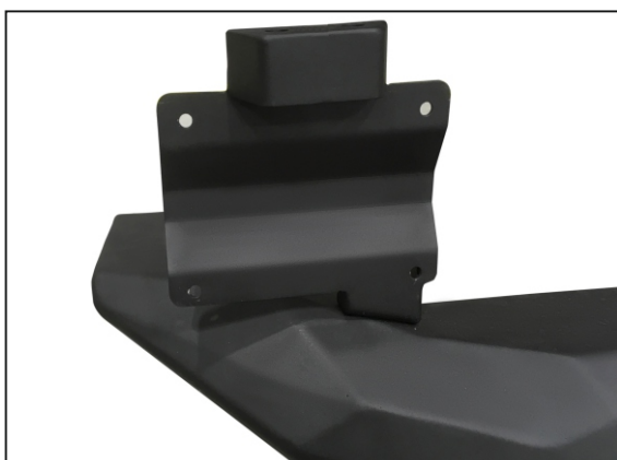
17. Install license plate bracket (pos.2) using screws M6x20 (pos.B), washers 6 (pos.H) and nuts M6 (pos.M). Torque hardware to * M6 - 9 Nm ( 6.6lb/ft).
