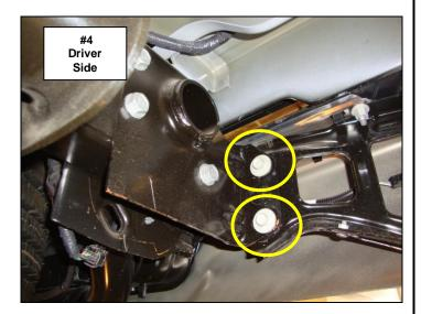
**Step 6** With Assistance, remove the factory bumper from the vehicle by rotating backwards to clear the boss located on the receiver hitch under the plastic center cover.
