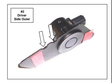
**Step-5** Prepare the inside of the replacement bumper surface where the bezel plates will be mounted with Isopropyl alcohol. A clean, dry surface is required in order for tape to stick properly.
