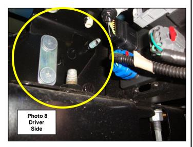
**Step-10** Remove the license plate, disconnect the license plate lights, and If equipped disconnect the backup sensors from the factory bumper wiring harness.
