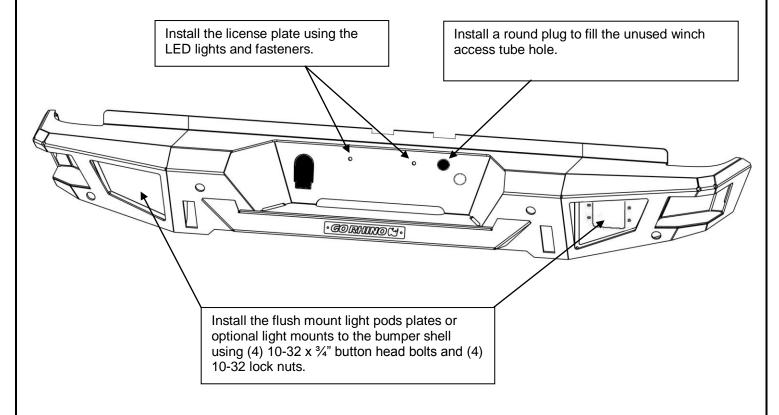
Step-15 Remember to check and retighten all factory and supplied nuts and bolts periodically.
