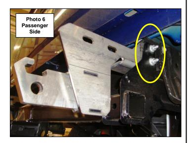
**Step-8** With assistance attach the bumper shell brackets to each frame bracket using (2) ½" x 1 ½" hex bolts, (4) ½" flat washers, (2) ½" lock washers and (2) ½" Hex nuts, Align the bumper shell with the vehicle, verify that the tailgate clears when lowered, and tighten all nuts and bolts, (Photo 7 & 8).
