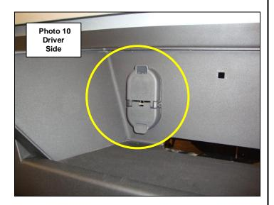
**Step-11** Reconnect the factory bumper wiring harness to the sensors and to the vehicle wiring harness.
