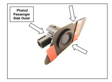
**Step-4** Prepare the inside surface of the bumper shell where the bezel plates will be mounted with Isopropyl alcohol. A clean, dry surface is required in order for tape to stick properly.
