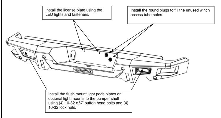
Step-16 Remember to check and retighten all factory and supplied nuts and bolts periodically.
