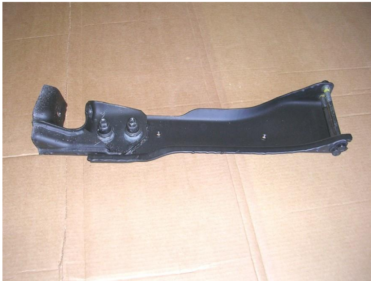
Figure 15: Factory crossmember and frame section removed.
