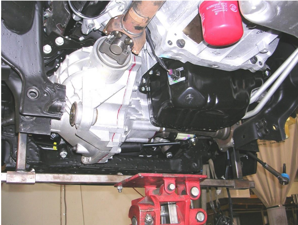
Figure 14: Factory crossmember and frame section removed.
