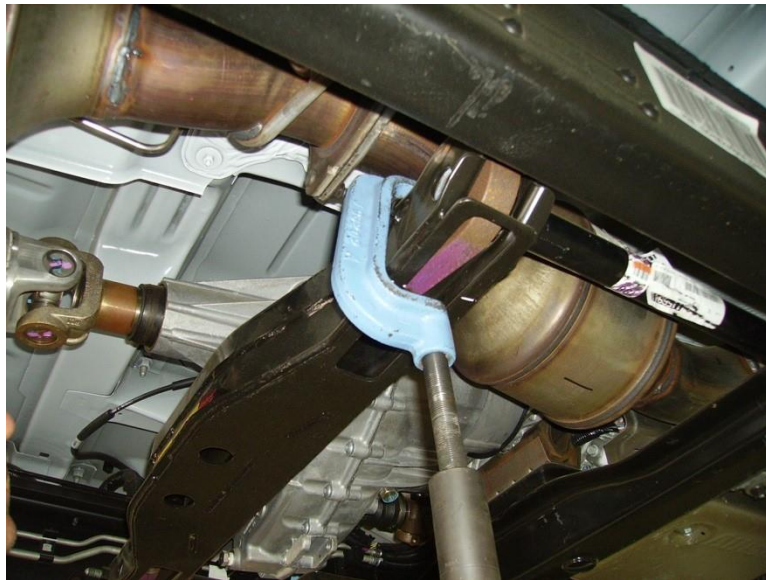
Figure 2: load torsion bar to remove adjuster nut
