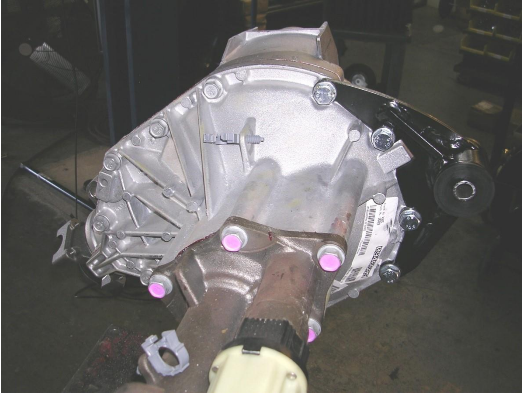
Figure 17: part #8151 Cognito Driver Side Differential Mounting Bracket installed
