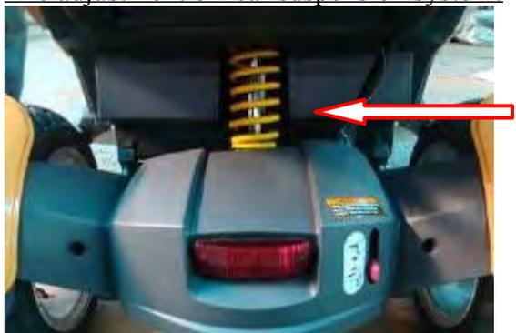
The softness of the rear suspension system is adjustable. There are altogether 5-level of adjustments. It is applicable with around 120kg and each level can bear up to 13.5 kg.
