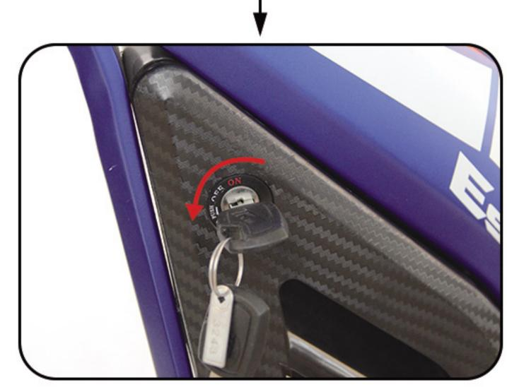
Press down the key and turn it counterclockwise to unlock your battery.
