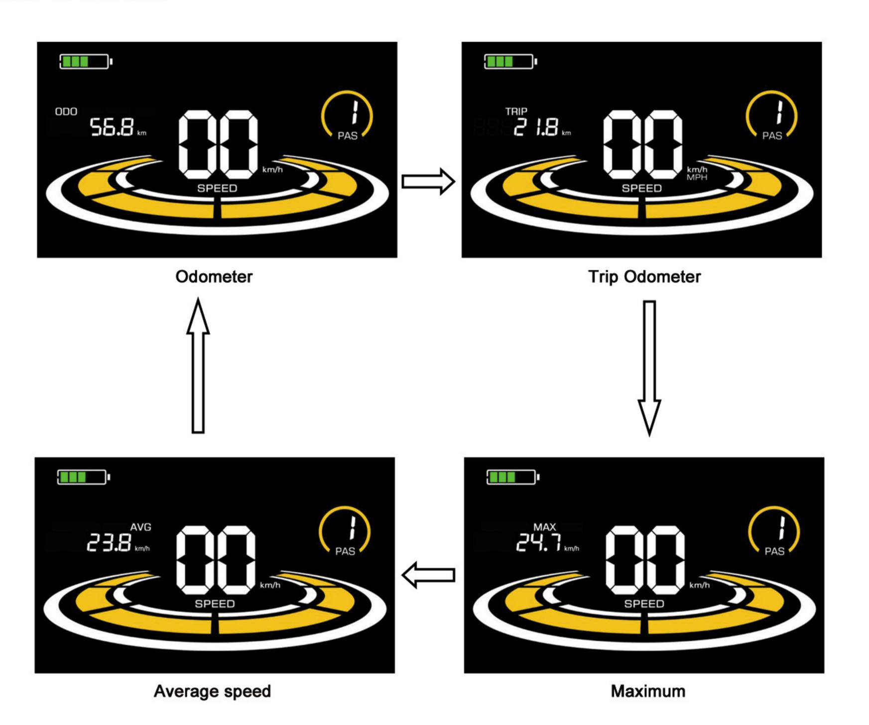
When the display is powered on, it will show the Current Speed (km/h) and Odometer (km) by default. Short press
