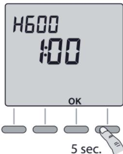
**CF01 – Correction of room temperature measurement.**
