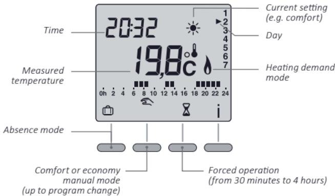
When starting up, the temperature measured by the thermostat is displayed (the symbol appears above the °C).
