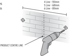
3. Drill four mounting holes with 10mm diameter x 50-60mm depth on the bracket wall side.
