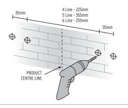
4. To install bracket, insert plastic plug into the hole and secure bracket with screws and tighten into position. Repeat to install second bracket.
