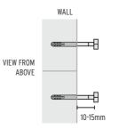
Align and locate cabinet mounting hole into screw and pull down slightly to secure correctly. Ensure unit is sitting flat and if required reduce distance of screw from the wall to suit.
