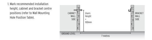
2. Drill two cabinet mounting holes with 10mm diameter x 50-60mm depth on the cabinet wall side.
