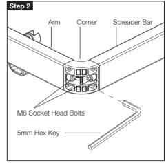
2. Loosen the M6 Socket Head Bolts using 5mm Hex Key and remove corner from Arm and Spreader Bar. Discard old Corner. NOTE: You may need to support the Spreader Bar until the new Corner is fitted.
