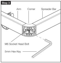
**3.** Secure by tightening the M6 Socket head bolts using 5mm Hex Key.
