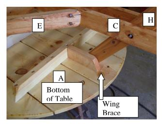
**Step 6:** Lay pre-assembled table top (**A**) upside down on a padded surface. Then secure the leg (**H**) to the wing brace of pre-assembled table top (**A**) using 4" lag bolt (**G**). Use  $\frac{1}{4}$ " washer (**W**) when fastening the lag bolt.
