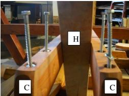
**Step 8:** Attach pre-assembled seat (**B**) to frame as shown (**C**). Align to back edge of the seat (**B**) with the ends of the braces (**C**), and measure to center the seat as much as possible. Use 4" lag bolts (**G**) through the pre-drilled holes in the braces (**C**) to secure. Use a ½" washer (**W**) when fastening the lag bolt. Note: Use a level to get the best alignment for the seat. Seats may still appear crooked at this point. This should be corrected in the next step.
