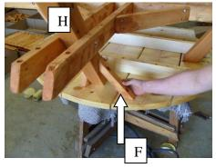
**Step 7:** Align and attach an 11" brace (**F**) to each side of each leg (**H**) securing it to the table bottom, using 2 ½" lag bolts (**I**). Use ¼" washer (**W**) when fastening the lag bolt. A total of 8 braces.
