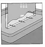
Capillary cementing. Apply solvent to inside edge.
