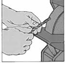
"Flats" ground into the cutting edge will prevent a drill bit from grabbing.
