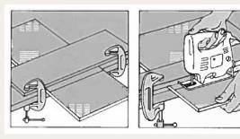
Clamp sheet firmly to table before cutting with a saber saw.
