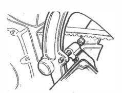
Side mount Plate Holder when using the HL passenger pegs.
