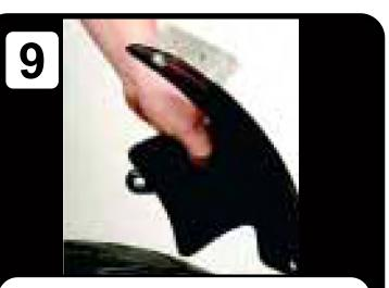
9. Attach the upper spacer to the new rock guard (slot facing down). Slide the new rock guard into place.
