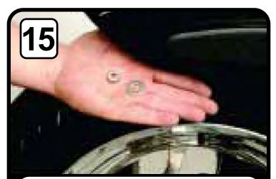
15. Using the hardware provided, put the washer on first, then the locknut. (No Loctite should be used to secure locknut).
