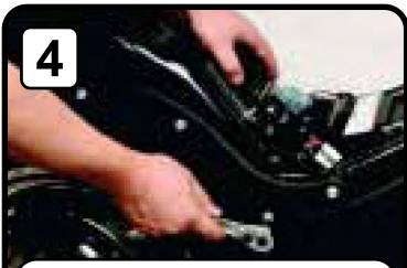
4. Remove the 4 strut cover bolts (2 on each side). Followed by the other 4 bolts holding the strut covers to the internal struts.
