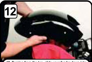
12. Coming from the top, slide your fender down into place. Note: Squeezing the fender might help sliding it into place.
