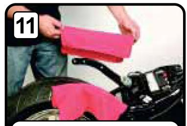
11. Cover the stock internal struts using a shop towel to prevent scratching your new paint.
