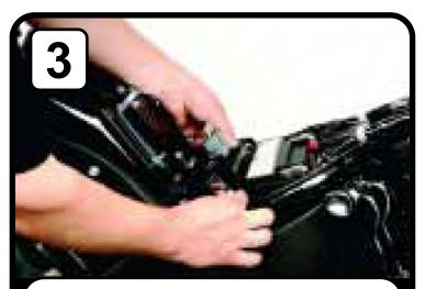
**3.** Disconnect your ECM unit and the T-signal/Tail lamp connector located to the right of the fuse box.
