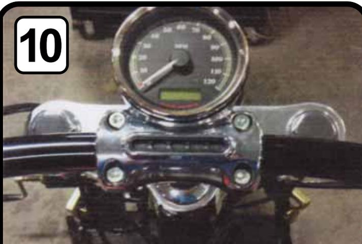
10. Now will be the time to install the riser spacers for extra clearance between handlebars and gas tank.
