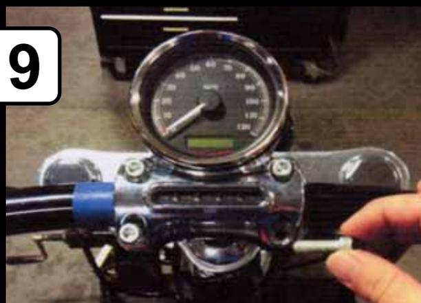
9. First re-install riser clamp and double-check that speedometer is centered. Next, double-check that dash indicator is facing the right way. Make sure that your marks on the handlebar and risers are lining up. Stock bolts will be used again. (Blue Loctite is recommended.)
