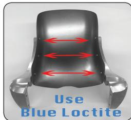
11. Install the Struts on to the Fender. Use Blue Loctite on all 6 Button Head Bolts.
