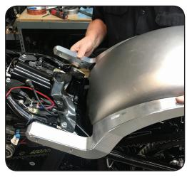
14. Mount the Strut-Fender Combo onto the Frame.
