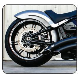
18. Remount Wheel and Brake Caliper.
