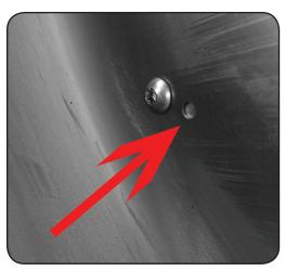
12. When using Light HL Bracktets. Run wire though fender hole and to strut wire channel.
