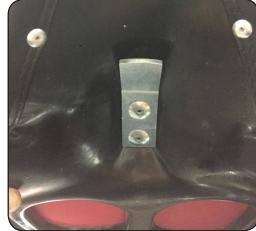
17. Mount and Place Solo seat in Place. Place seat Tongue in Frame in front and push down on Center of seat to place in correct location, then push on back to set the suction cup.
