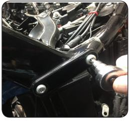
3. Remove that Rear Fender by unbolting the Fender Strut Bolts on each side. Both Fender and Struts come off together.
