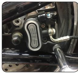
4. Remove the Rear Brake Caliper, use 12mm socket. And Note where the ABS sencor wire is located for re assembly.
