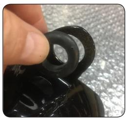
7. Install the Rubber Gromets into brackets on Rock Guard. Spray a little Windex on the Gromets to make it slide in easier.
