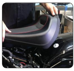
1. With bike properly secured for repair. Remove Seat
