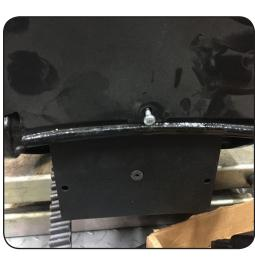
5. Remove that Plastic Spash Guard with single screw. Re-use this screw later.
