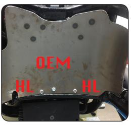
10. Bolt Rock Guard to Swing Arm using stock OEM Screw and Two Supplied Screws. Center uses OEM Screw, outer use Supplied Screw
