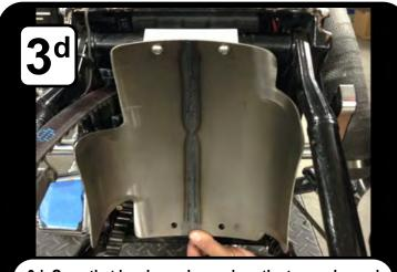
3d. Once that has been done, place the top rockguard spacer over the steel tab on the swingarm and push down to secure.
