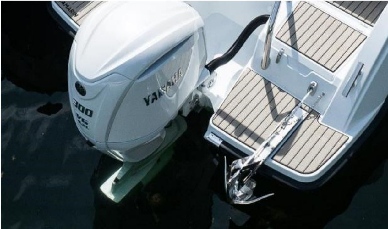
Anchor winch aft
