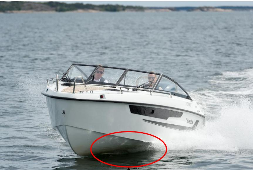
Negative chines make the boat very stable and the driving experience well-balanced, forcing the water spray wider to the sides
