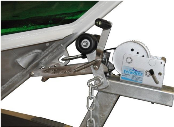
Lever handle up - Engaged.
