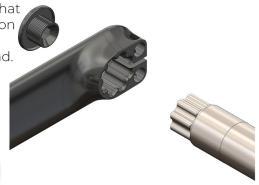
4. The pedal inserts (part 7) can now be installed. Ensuring the DS pedal is a standard thread and the NDS pedal is the LH thread, this is denoted on the pedal insert, the insert is positioned from the reverse side of the arm.
