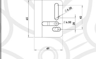
front and rear bolts of the adjustable riser in step 3 (42mm centres) rather than the two centrally tapped holes (25mm centres). With this set up, you would need to replace the M5x18mm and M5x25mm low cap head bolts in the adjustable riser with M5x30mm and M5x35mm countersunk head bolts. WattShop does not supply these bolts. In this arrangement your armrests will need to accommodate a 42mm fore-aft bolt hole centre.
