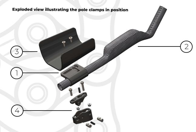
Ideally the pole clamps are paired with our adjustable angled risers but can also be used as a standalone item. Although in the latter arrangement mounting options need to be considered.
