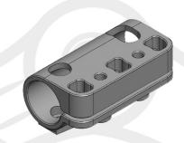
3. Position the pole clamps on top of the adjustable riser, locate the M5x22mm low cap head into the rear holes (part 2) and the M5x30mm low cap head into the front holes (part 3).
