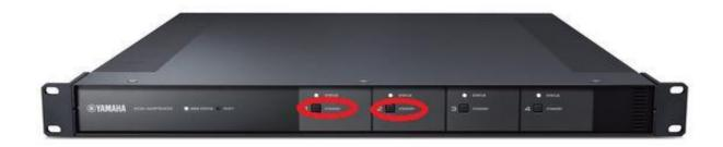
Set all Zones to standby and then hold down the 'CONNECT' and 'CONNECT2' keys simultaneously for 5 seconds or longer.
