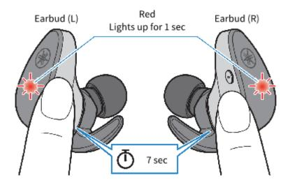
3: After the power turns off, hold down the function key and the – (minus) key for 10 seconds. Make sure that the indicator lights up as shown below.
