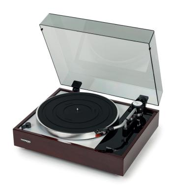
In 1965, the Thorens TD 150, an inconspicuous little turntable, came on the market and thus started a technical revolution in record player manufacturing. For the first time, a spring-suspended sub-chassis with an inner platter driven by a flat belt was used in a mass-produced unit. The principle proved to be very successful and found many imitators in the years since.
