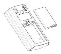
Press down on the belt clip to release it. Remove the battery cover and insert the battery as shown in the diagram. Replace the battery cover and belt clip.
