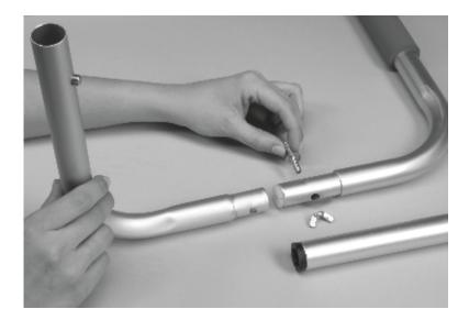
Attach elbow to arm as shown using bolt with washer and wing no Repeat with other side.
