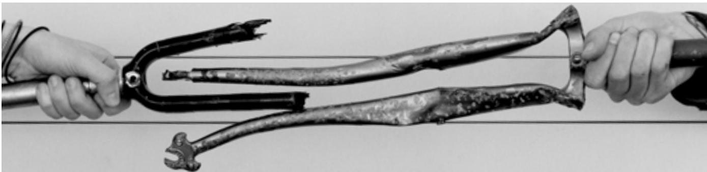
This carbon fork died in a sword fight with a steel fork that (in that fight) was barely scuffed. The mangled steel fork here died in Taichung, when a box of forks fell off a truck when the driver swerved to miss a wayward dog. The dog was fine, but this fork got run over by several cars. Although neither fork was killed during riding, both show how carbon and steel respond to stress.
