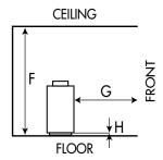
Clearances can be reduced with shielding acceptable to local authorities. Reduced installation must comply with NFPA 211 or CAN/CSA-B365.
