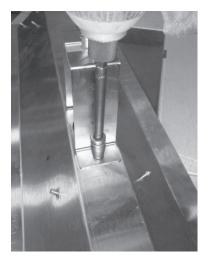
Figure 5.2 Attach Flexible Bulk Head and Bracket to Pan
