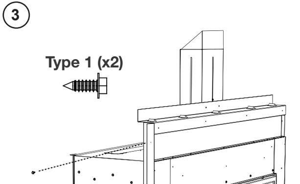
Secure with screw supplied in the manual baggie to the upper front frame
