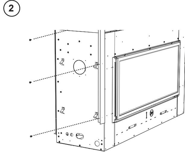
Align the nailing tab with the hole on the appliance then secure with the screws removed in step 1.
