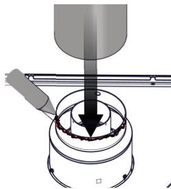
USE RED SILICONE TO SEAL REDUCER TO THE AIR INTAKE COLLARS.
