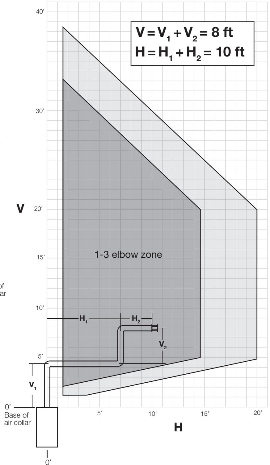
**V and H are measured from the center of the vent elbows**
