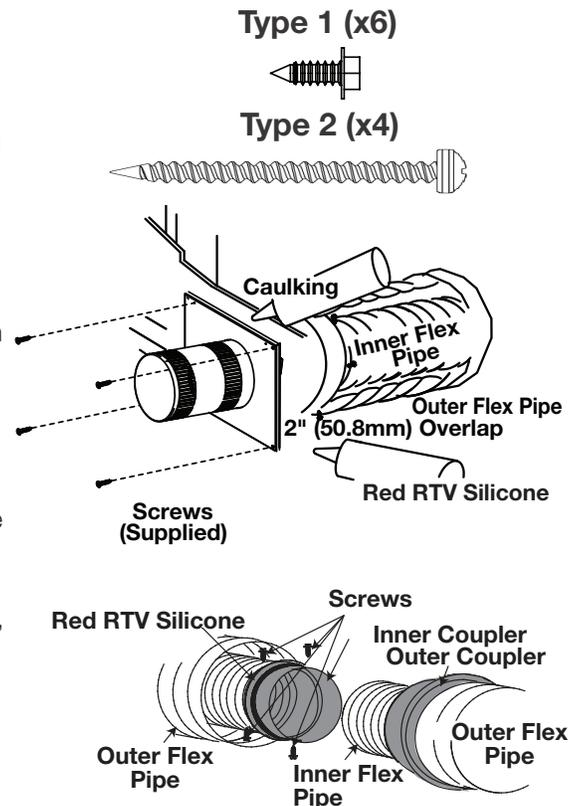
**The air terminal mounting plate may be recessed into the exterior wall or siding no greater than the depth of its return flange.**
