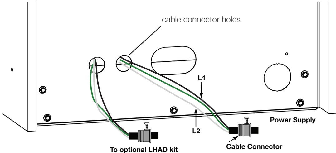
Route power supply and optional LHAD (Linear Hot Air Distribution) kit through the outer firebox to the receptacle mounted on the bottom of the appliance. For optional LHAD kit installation, please refer to the leaflet provided in the kit.
