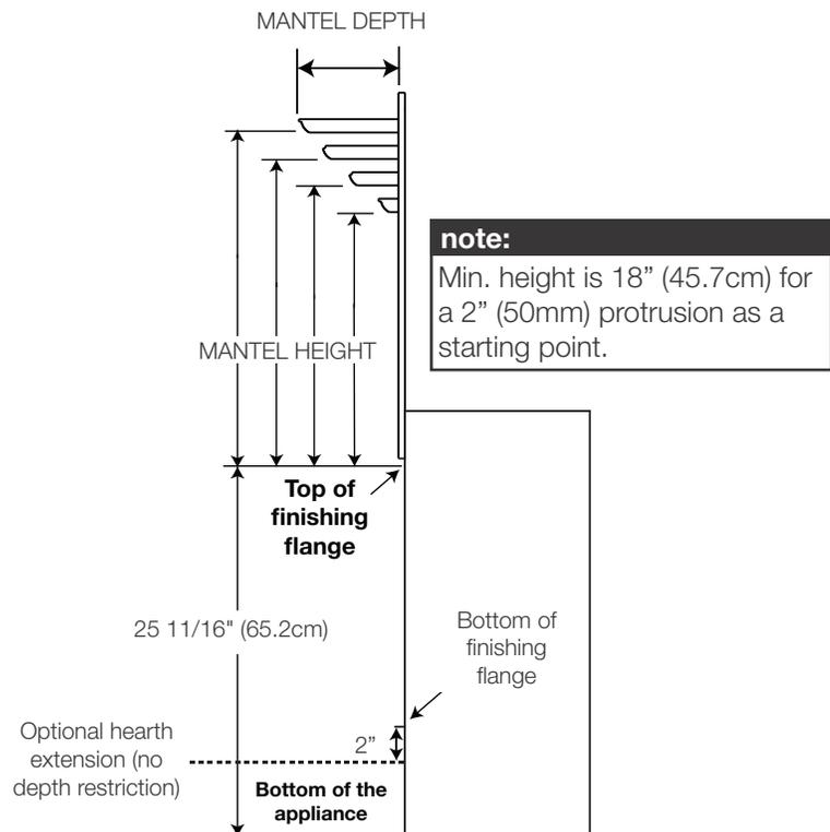
Installing a mantel between this appliance and electronics or other materials that may be sensitive to heat will reduce the effect of direct heat on them.
