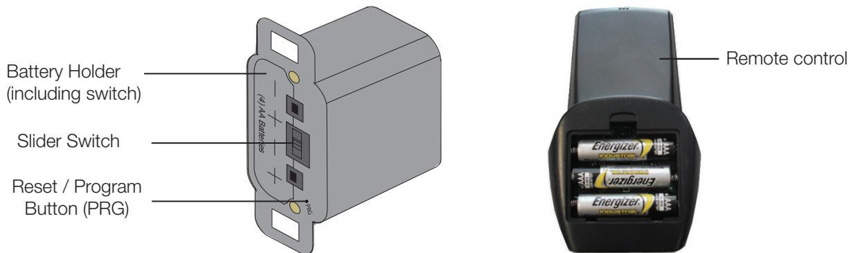
Receiver must be located within 8 feet (2.4m) of this side of the appliance and must be accessible for programming the remote.
