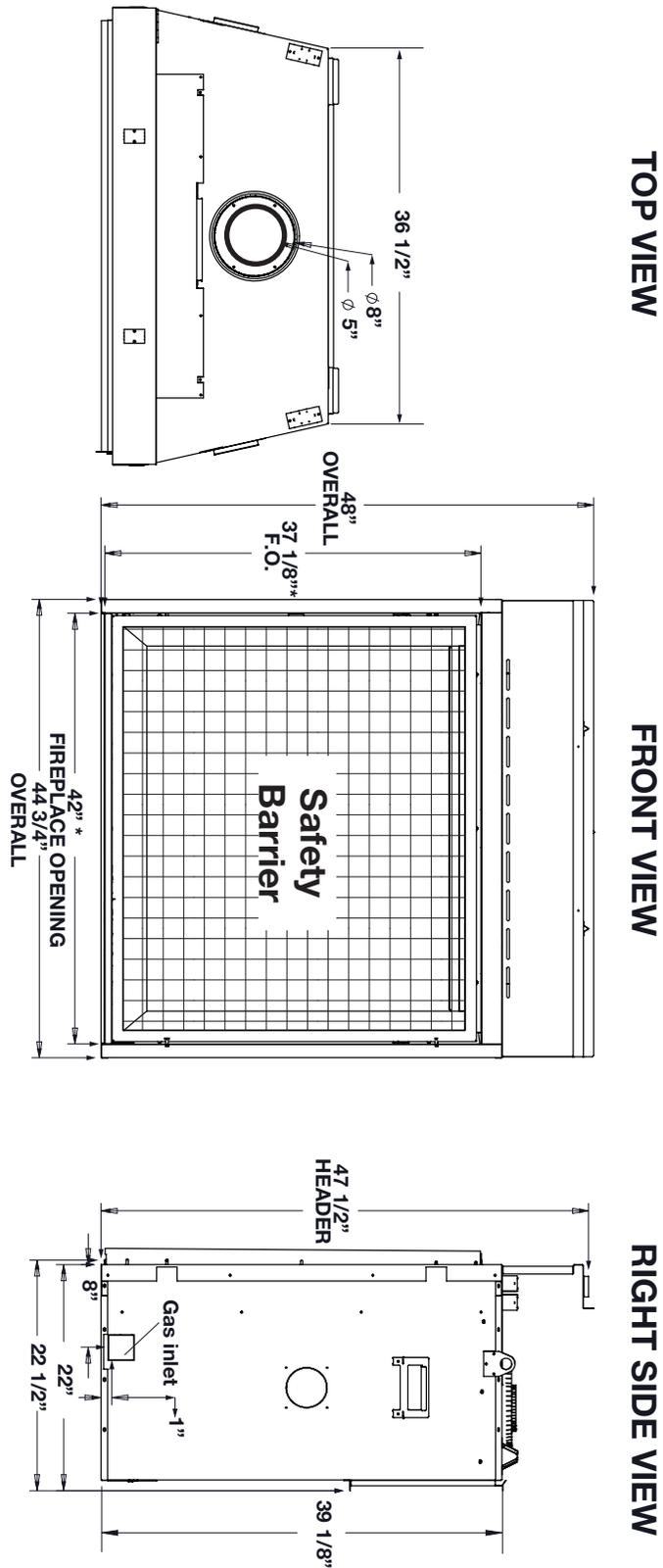
\* Finishing flange (the finishing flange defines the perimeter of the fireplace opening. Framing or finishing materials must **NEVER** encroach inside the finishing flange).
