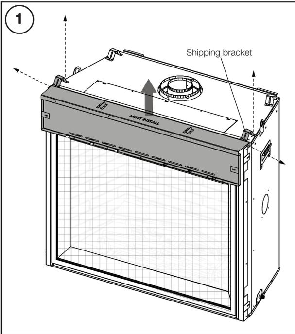
Remove the 4 screws securing the header shield.
