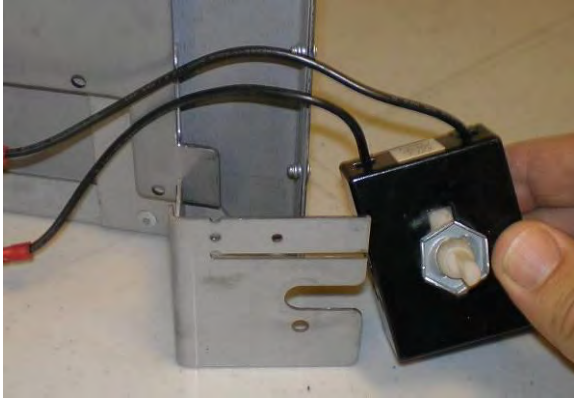
1 Remove Fan Control Switch From Current Position.
