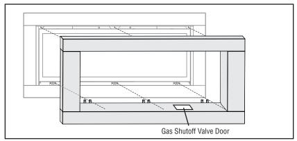
Figure 42 - Noncombustible Material with Bezel and Barrier
