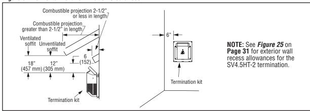
Table 7 - Horizontal vent termination clearances for buildings with combustible and noncumbustible exteriors
