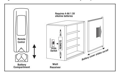
Figure 44 - Remote Control Transmitter
