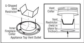
Figure 13 - Vent restrictor assembly
