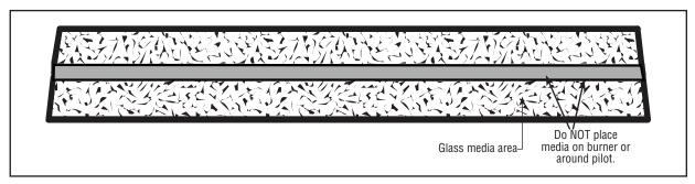
**NOTE:** It is important to ensure proper media placement per the manual when installing these units. Verify pilot flame is not obstructed. Ensure media does not fall through the pilot hole in the floor. See Verifying Appliance Operation on **Page 38**.
