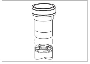
**12. Install the vertical termination**—Extend the vent sections to the correct height (*Table 6*). The SV4.5CGV-1 Vertical Termination (*Figure 21*) installs in the exact same fashion as any other Secure Vent® section.
