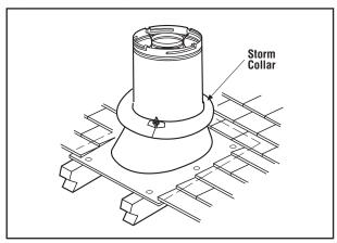
Figure 21 - Installing the Vertical Termination
