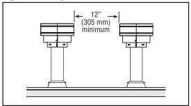
Terminate single vent caps relative to building components according to **Table 6** and **Figure 4**.
