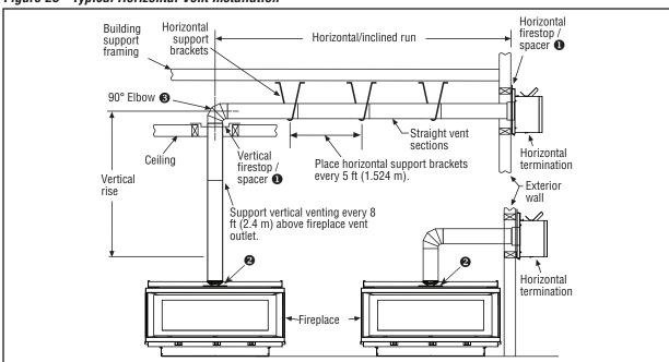
Figure 23 - Typical Horizontal Vent Installation
