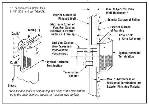
Table 21 - Venting Components Required for Various Exterior Wall Thicknesses, when using Typical Termination Kits
