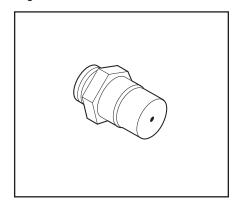
**14.** Apply pipe joint compound or Teflon® tape to all pipe fittings before installing.
