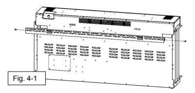
• After you have selected a suitable location for wall mounting, locate the studs on the wall. You must be able to secure to a minimum of 2 studs for proper installation of the bracket.
