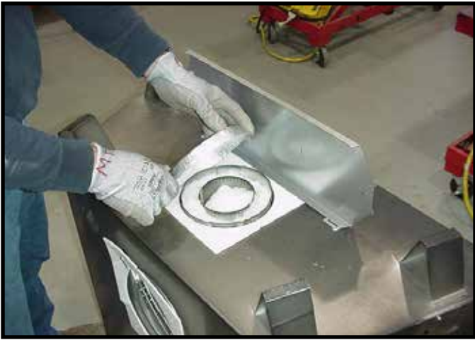
Figure 6.8 Remove the seal cap.
