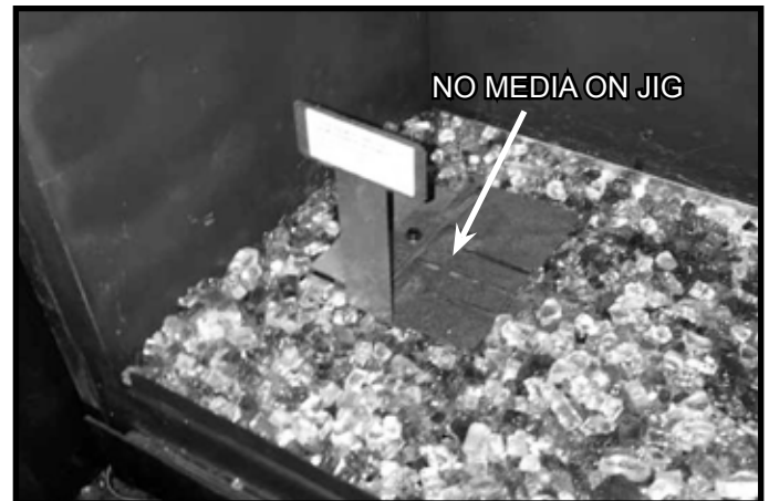
Figure 2. Media Placement Jig in Place
