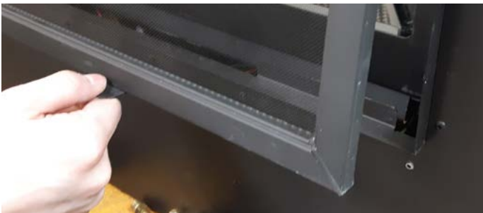
Figure 20.b Lift out the Retaining Tabs and screen
