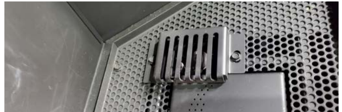
Figure 13. Removal of pilot cover
