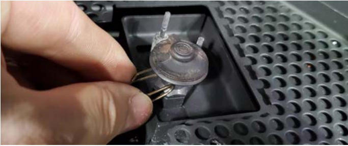
Figure 13.d Removing the spring clip
