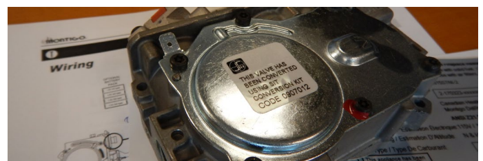
Figure 13.k Conversion label on valve
