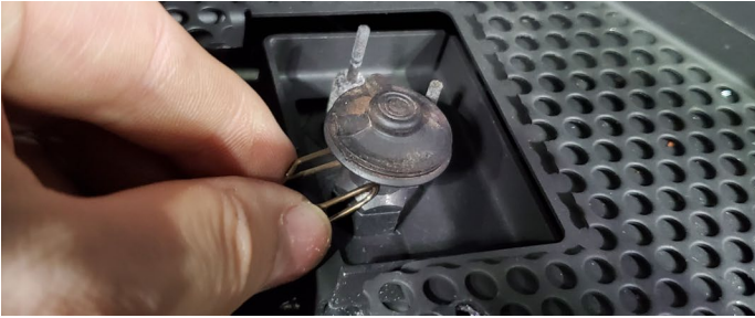
Figure 13.d Removing the spring clip
