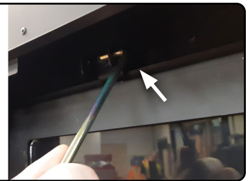
Figure 21.d Pull door latches
