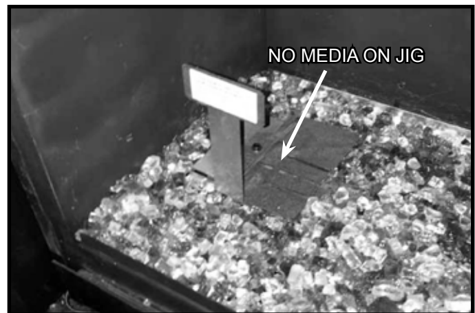
Figure 2. Media Placement Jig in Place
