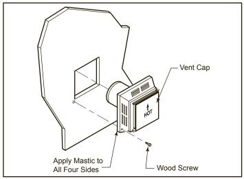
Figure 16 - Install Horizontal Vent Cap
