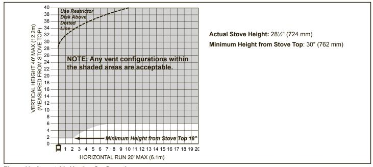
Figure 11 - Acceptable Venting Configurations
