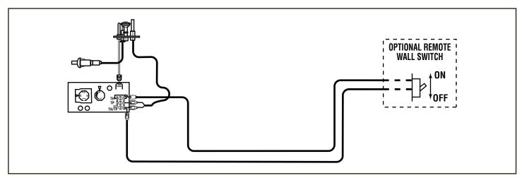
Figure 33 - Wiring Diagram for Wall Switch
