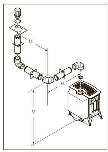
Figure 27 - Vertical Rigid Venting Configuration using Three (3)  $90^\circ$  Elbows with Two (2) Horizontal Runs
