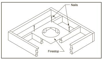
Figure 23 - If area above is a room, install firestop above framed hole as shown
