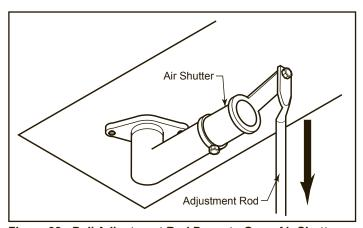
Figure 38 - Pull Adjustment Rod Down to Open Air Shutter
