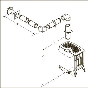
Figure 19 - Horizontal Termination Configuration for Rigid Venting Using Two (2) 90° Elbows
