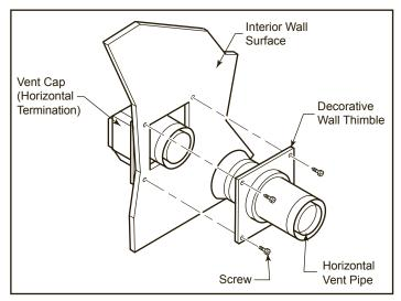
Figure 18 - Connect Vent Cap with Horizontal Vent Pipe
