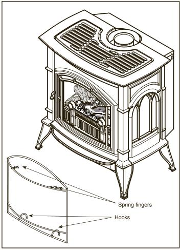
Figure 36 - Safety Barrier Installation
