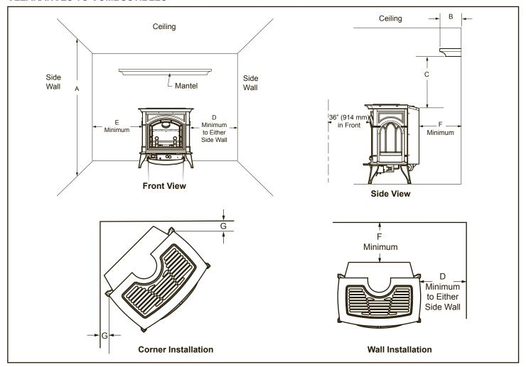
Figure 4 - Minimum Clearances to Walls and Ceiling
