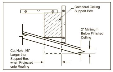
Figure 25 - Cathedral Ceiling Support Box Installation
