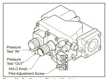
Figure 32 - Gas Pressure Check at Gas Valve
