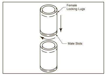
Figure 14 - Rigid Vent Pipe Connections
