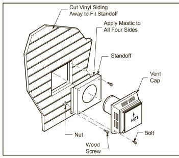
Figure 17 - Install Vinyl Siding Standoff
