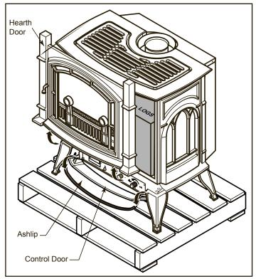
Figure 7 - Open Control Door and Remove Hearth Door
