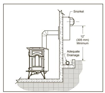
Figure 13 - Snorkel Termination with Drainage Pipe
