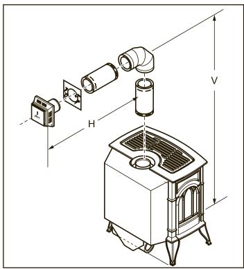
Figure 18 - Horizontal Termination Configuration for Rigid Venting Using One (1) 90° Elbow
