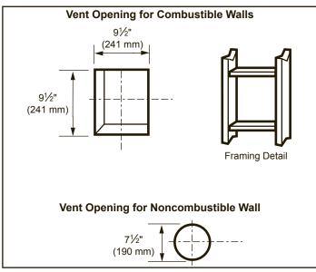
Figure 15 - Locate Vent Opening on Wall
