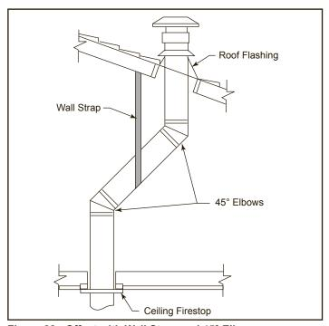
Figure 22 - Offset with Wall Strap and 45° Elbows
