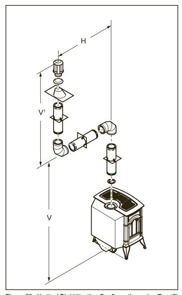
Figure 28 - Vertical Rigid Venting Configuration using Two (2)  $90^{\circ}$  Elbows
