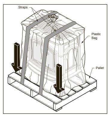
Figure 6 - Remove Straps and Plastic from Unit
