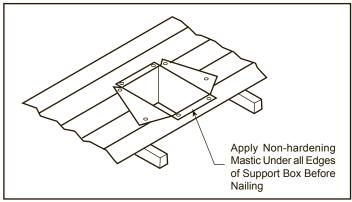
Figure 26 - Installed Cathedral Ceiling Support Box
