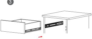
Insert drawer into cabinet and shut drawer to engage slides.
